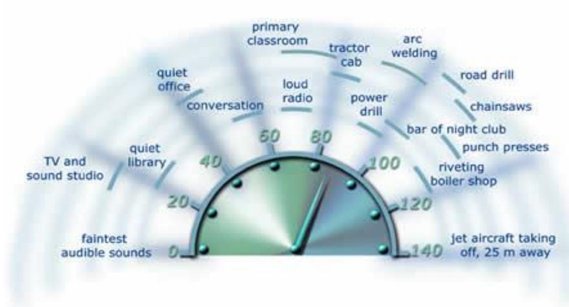
To assist in determining noise levels a basic rule of thumb can be applied:
